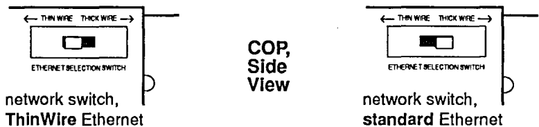
Figure 3: Network Selector Switch, OGA Board COP
